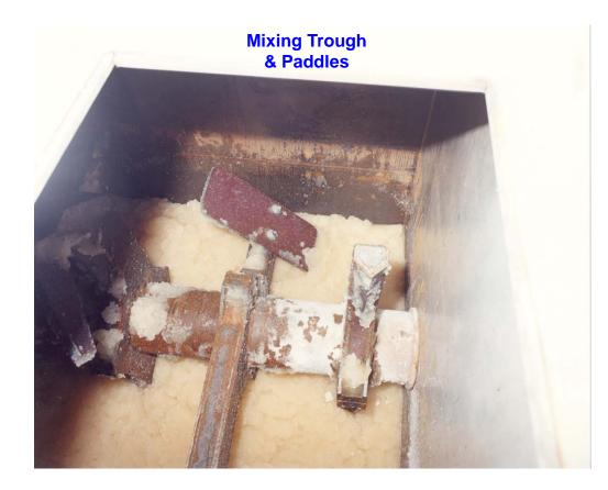
The trough was filled with 1,100 gallon of waste liquid, the mixing paddles started and reactants and polymer were added gradually during the mixing.
