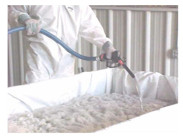
In this step-by-step/layered approach, the entire liquid content of the B-25 box is solidified to meet EPA Paint Filter Test Requirement.
