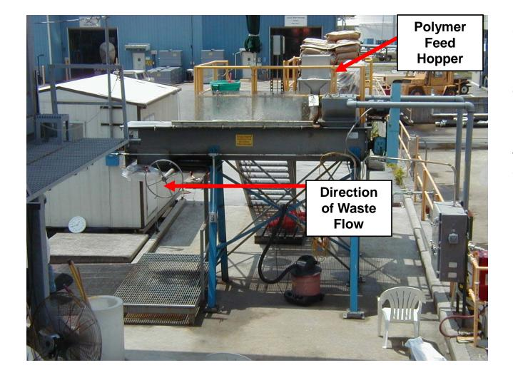
Above this large screw auger was a platform with a small hopper equipped with a small metering screw to add polymer sorbent to the large horizontal auger at a controlled rate.
