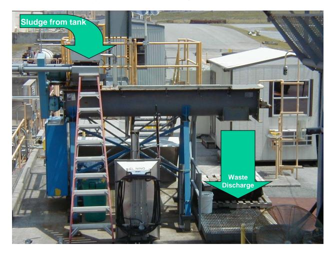
The sludge was pumped from the tank into one end of a horizontal screw conveyer/auger.
