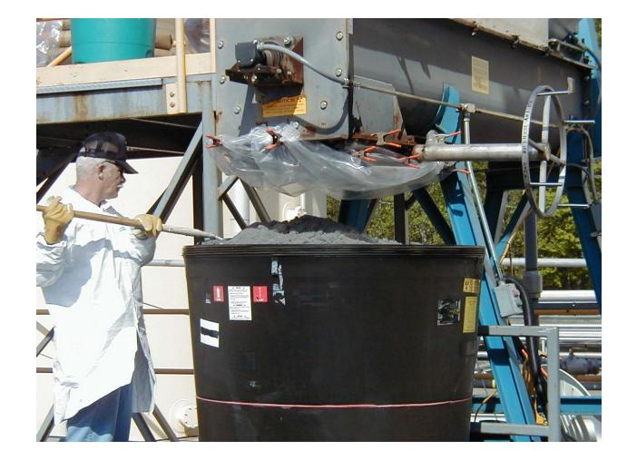
The polymer mixed very efficiently with the sludge as it moved down the long auger.
