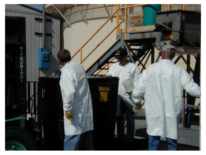
The lined, 21<sup>st</sup> Century containers were then sealed and shipped to Utah for land disposal. The operation processed 600,00 to 800,000 kgs/year of sludge.
