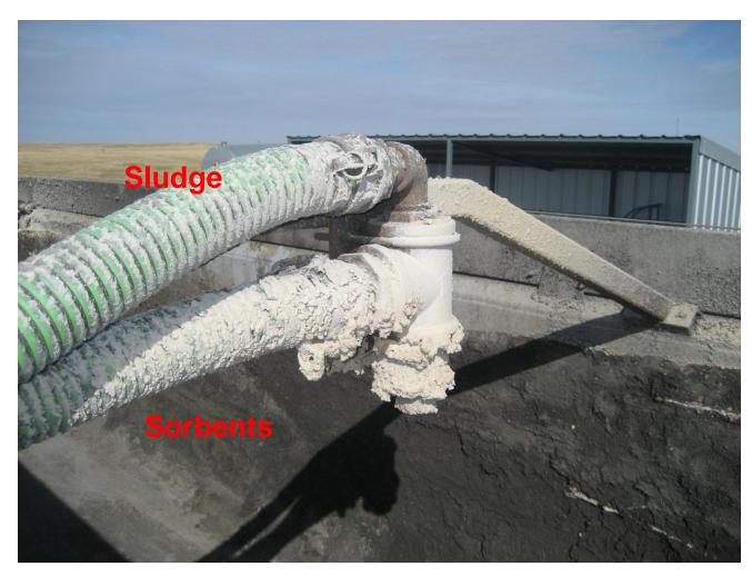
The sludge is pumped to the top of the truck where the liquid meets the dry sorbent through this L-shaped valve.
