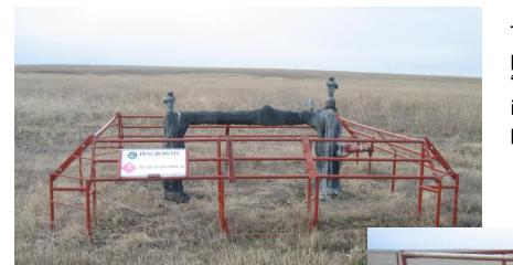
To maintain the flow of gas, wells are periodically subjected to a treatment called "Swabbing." High pressure brine water is injected into the well to crack and re-open plugged fissures so that the gas flows easily.
