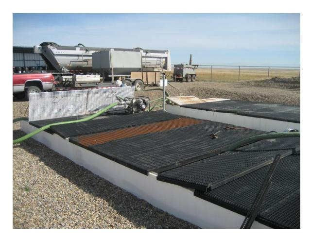
The swabbing waste liquid is pulled from the well formation into vacuum trucks and then deposited in pits where the solids settle out.
